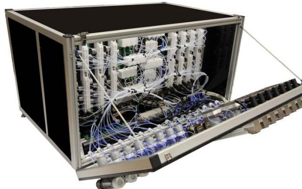
**Special valves** are located in the main stream flow. This ensures continuous washing of the odorant residues and only negligible dead space. After activation the odour flow its concentration stabilizes after 0.5-1 sec.
